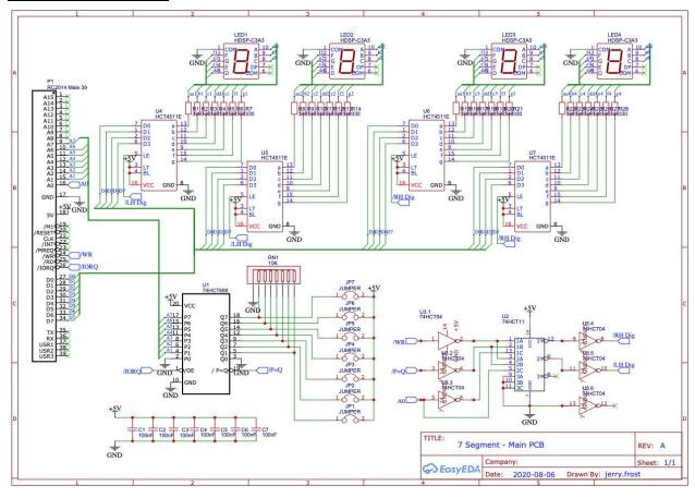
JP1-7 are used to set the address of the upper 7 address bits (A1 to A7). When the address bus matches this, U1 sends a "/P=Q'' signal to U2. If the "/WR'' write signal is also low, then U2 will enable either U4 and U5, or U6 and U7 depending on whether the lower (A0) address bit is a 1 or a 0.
