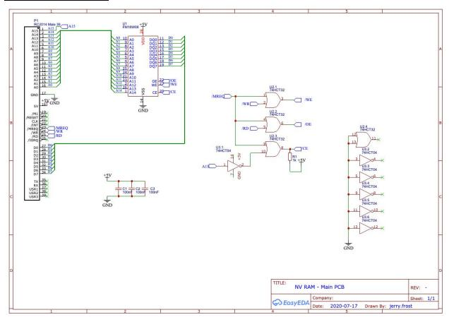
U1 is the F-RAM IC, and is connected directly to the RC2014 data bus, and A0 to A14 of the address bus.
